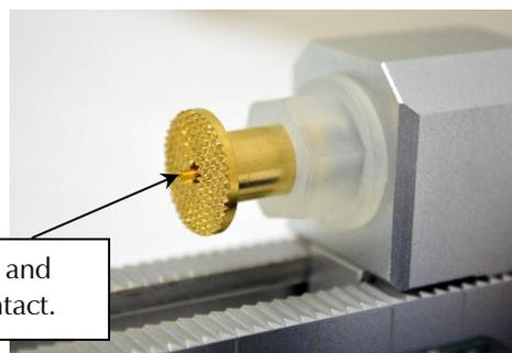
The central pin is independent of and isolated from the surrounding contact.
