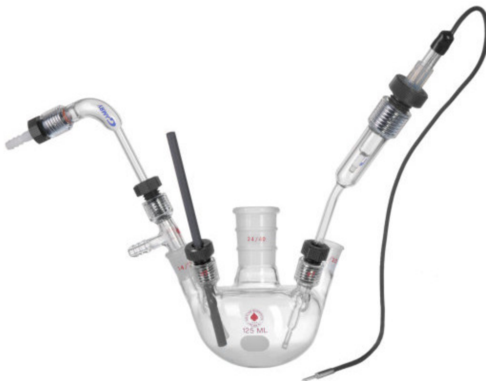
Figure 1. The Standard Configuration of a RDE Cell.
