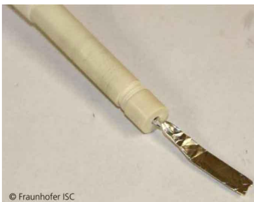
Fig. 4. 935-00084 assembled with foil electrode.
